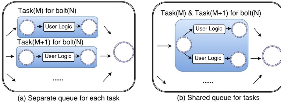
Figure 3.3: Modified Concurrency Model of Worker Process. (a) Default (original): Each task has an independent input buffer. (b) Modified: Different tasks, inside the same worker process, of the same operator (whose input only consists of shuffle grouping streams) share the input buffer.
