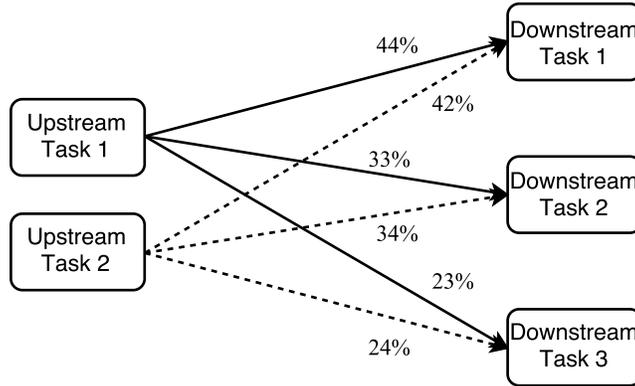
Figure 4.2: Asynchronous, Independent Load Adjustment of Upstream Tasks. The upstream tasks perform load adjustment at different moments, and they make slightly different decisions. 44%, 33% and 23% of upstream task1’s outgoing traffic are fed into downstream task1, 2, 3 respectively. 42%, 34% and 24% of upstream task2’s outgoing traffic are fed into downstream task1, 2, 3 respectively.
